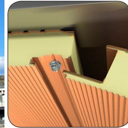
The perfect configuration of the joint makes the surface of the building envelope pleasant and uniform, and allows the panel to considerably reduce thermal bridges which, as it is known, cause energy dispersion and the formation of condensation.
